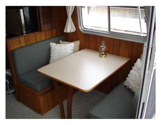
Transforming from dining to sleeping takes only a few moments. The table is lifted at the wall end from its (original Alwest) support ledge and placed on the rails along the fronts of the seats.
