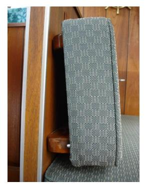
A key change to the forward seating area on Catherine Ann is the addition of reinforcing pieces behind/under the seat backs.
