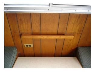
Tipping the table vertical causes the hinged leg to drop to its stored position where it is fastened with a strap and snap.
