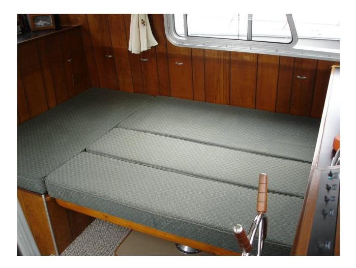
Pins in the outer seatback \_\_\_\_\_\_ section locate into drilled holes in the rails, to prevent the bed sections from sliding out of position
