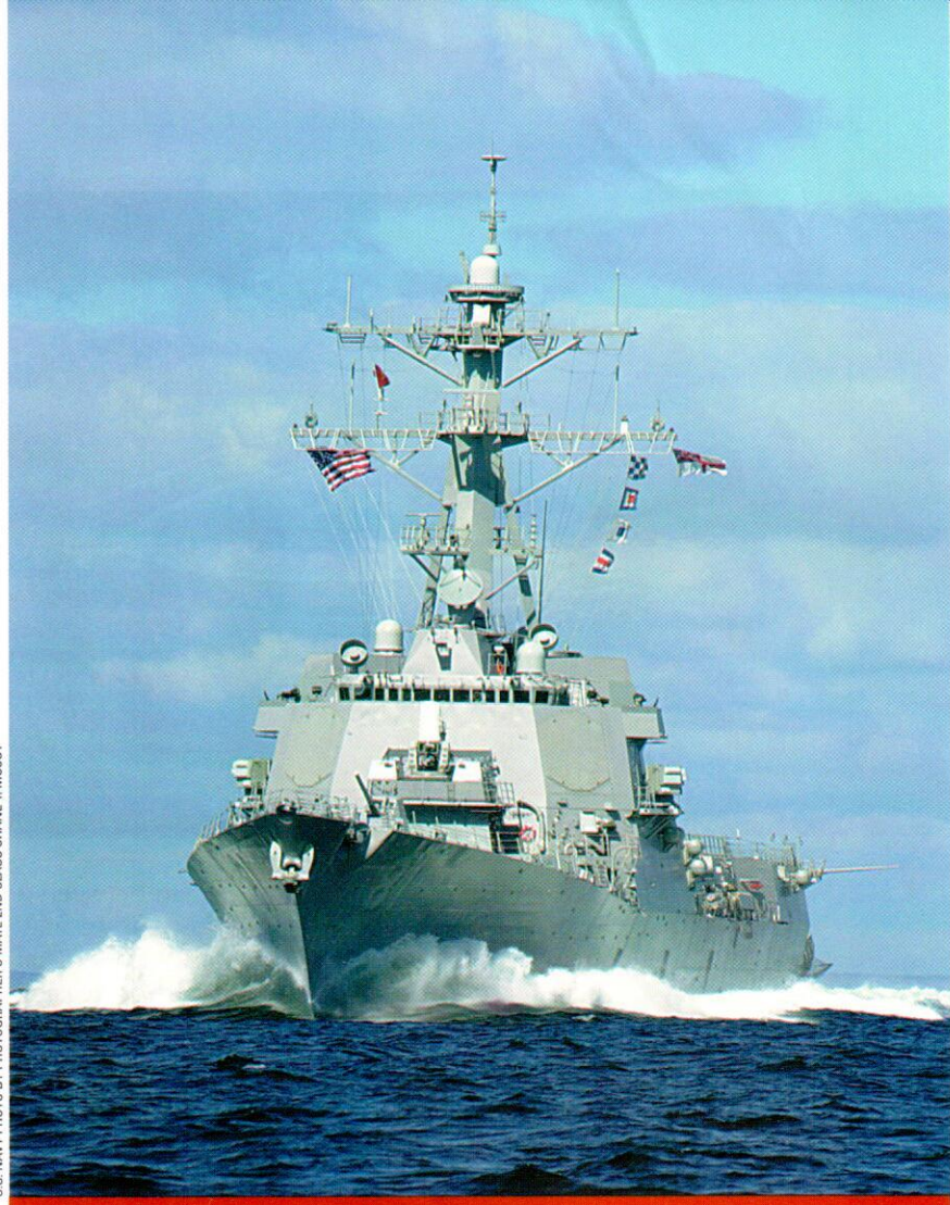
USS Winston S. Churchill (DDG 81) making a high-speed run in the English Channel. The Arleigh Burke-class destroyer with the Aegis weapon system is 510 feet long and carries 380 crew. This ship operates well beyond traditional speed-length ratios.
