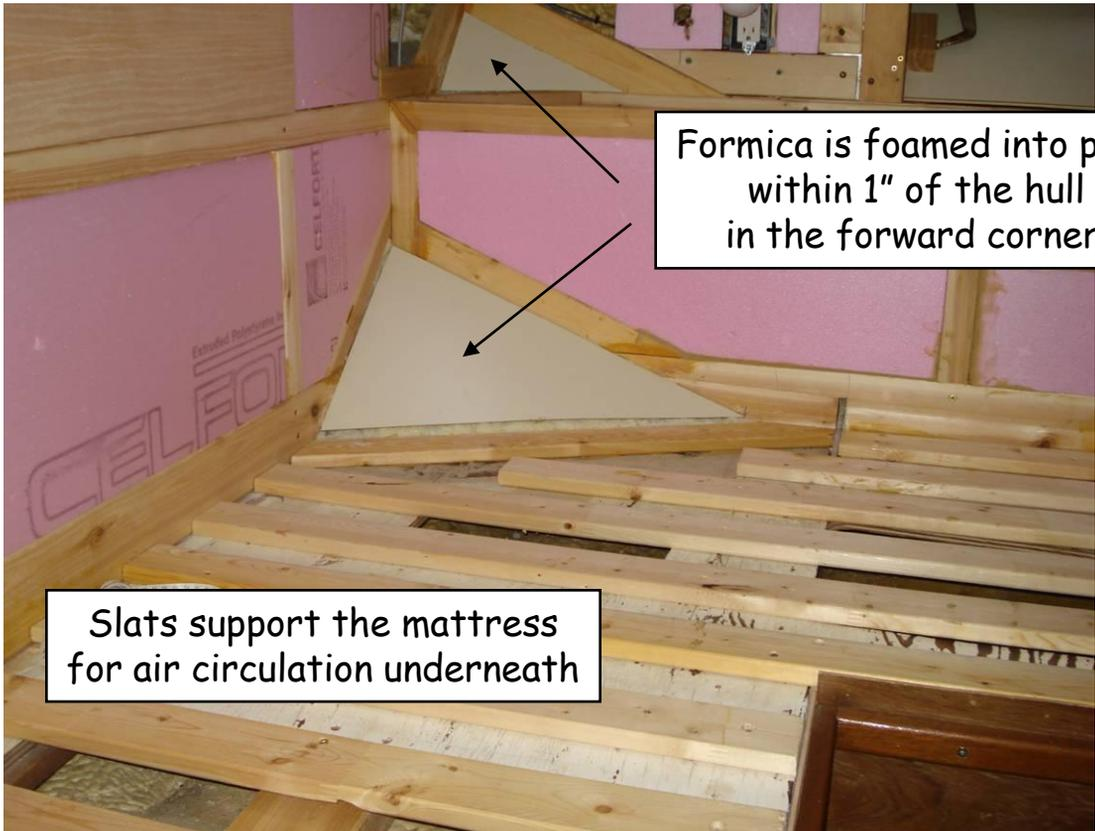
Formica is foamed into place within 1" of the hull in the forward corners
