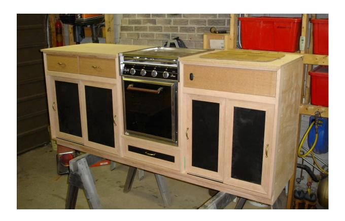
The new lower doors are side sliders to prevent opening when bumped or while underway. Micro switches turn on internal lights when the doors are opened.
