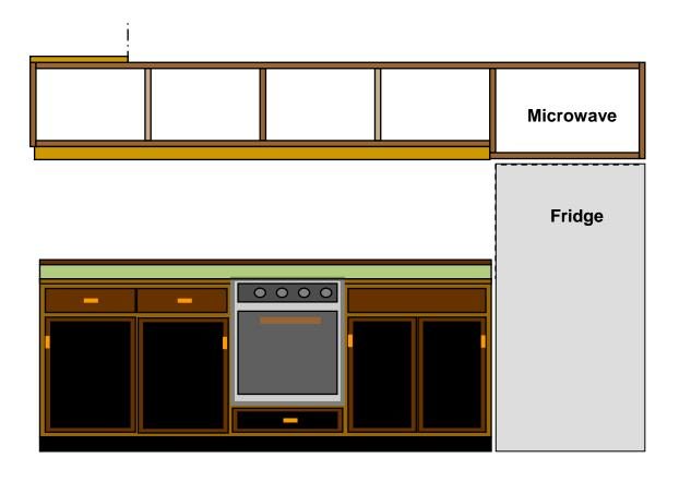
The new galley was fabricated at home, over the winter, in a "take-apart" manner (modeled after IKEA) so that the pieces would fit through the cabin door and could be reassembled at installation.
