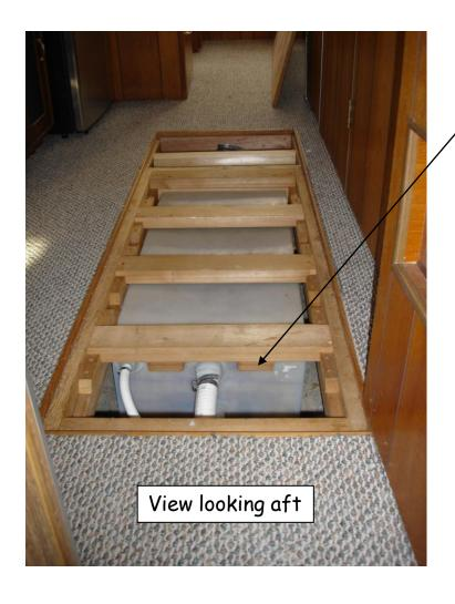
Note also that the forward removable crosspiece has two blocks on the underside to keep the tank from sliding forward.
