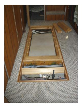
The first step was to extend the existing bilge access (in front of the fridge) all the way forward to open up the main bilge area.
