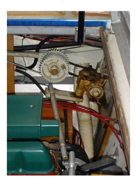
As the basics of the new system, I selected two Teleflex Sea Star HH5271 helm pumps and the Teleflex HC 5314 actuating cylinder. This combination has proven to be quite capable of steering the original twin Volvo 270 outdrives which do not have any power assist.
