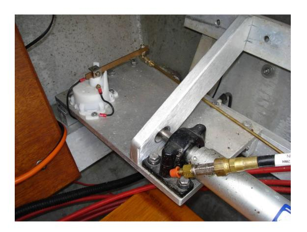
Since the hydraulic piping is fixed and the actuating cylinder articulates (a small amount) short sections of appropriate hydraulic hose are required to make sure that the hydraulic connections to the cylinder do not work loose. These hoses are available by special order from Teleflex for about \$50 each (or at the local hydraulic supplier for about \$10 each).
