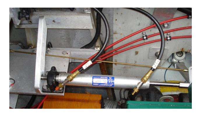
To plumb all this together, I chose to use the Sea Star recommended 3/8" soft copper (also known as refrigeration copper) tubing. The main reason for using this type of copper tubing is that it can be shaped by hand and can be bent back and forth (a few times) which is necessary to snake these tubes through the boat from cylinder to helm pump. Commercially available in 50 ft coils, this tubing does not have to be purchased from a marine supplier.
