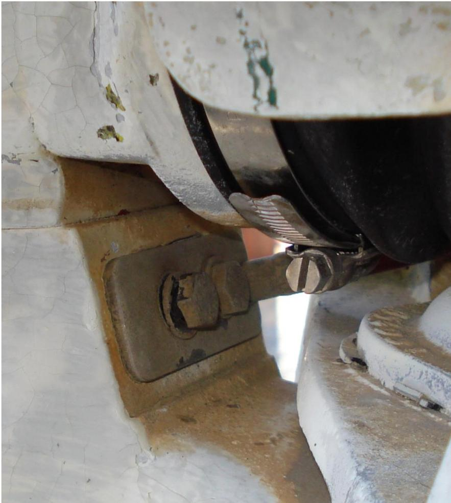
From inside boat, pull shift cable back through outer hose until it is completely free of outdrive. Don't pull any further than necessary.
