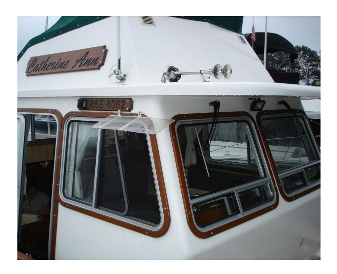
At an angle of about 45 degrees these will protect the window for its entire height, in all but the heaviest downpours or cross winds.
