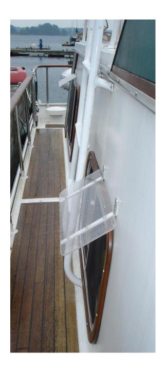
Each awning is made from 3/16" clear Plexiglas and is about 8" wide by the width of the window opening plus a few inches on each end.
