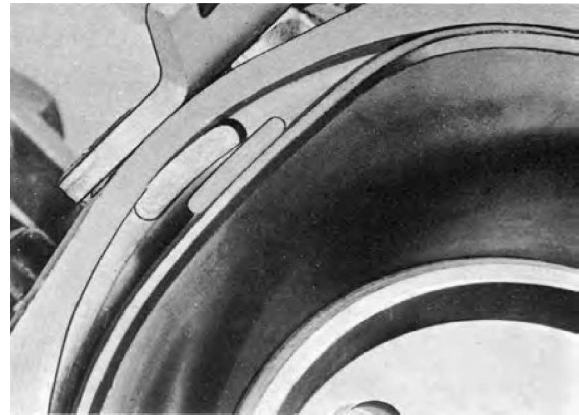
Fig. F3. Diaphragm location in carburetor body
