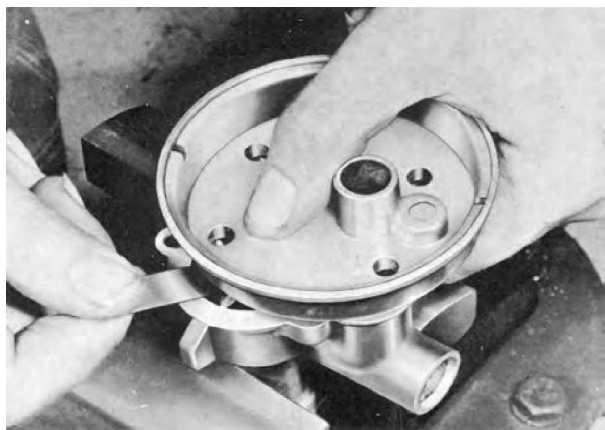
Fig. D8. Measuring the axial clearance
