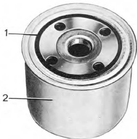
Fig. D4. Oil filter ready for fitting 1. Gasket (oiled) 2. Filter
