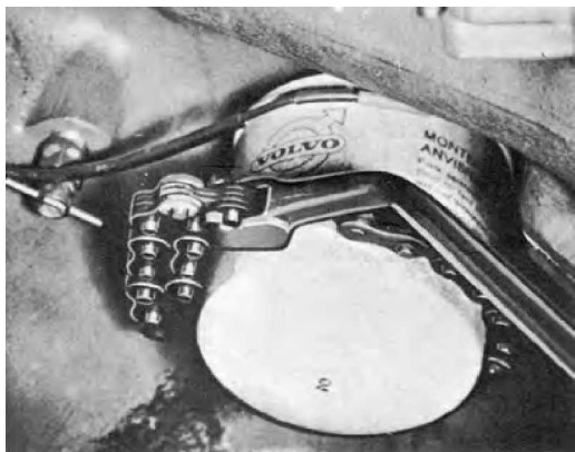
Fig. D5. Removing the oil filter
