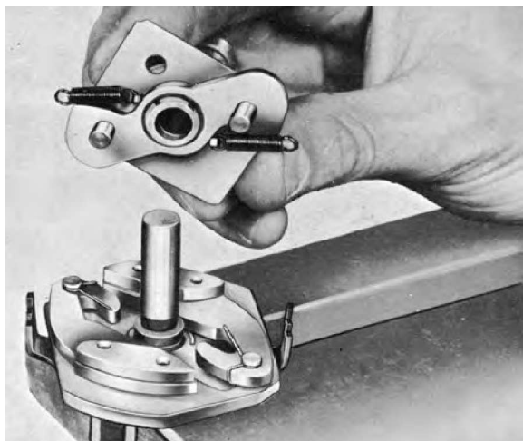
Fig. H5. Fitting the breaker cam
