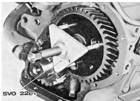
Fig. C12. Removing the camshaft drive (4-cyl. engine)
