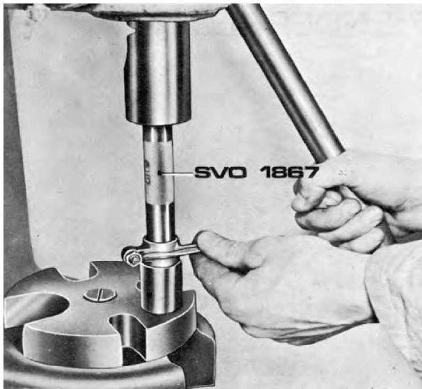
Fig. B6. Replacing bush in rocker arm
