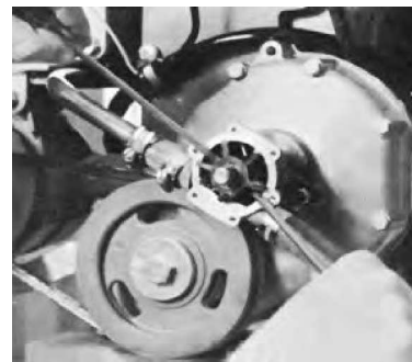
Fig. G 5. Removing the pump gear
