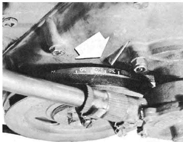
Fig. H6. Graduation for firing position (4-cyl. engine)
